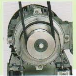
Schleifband Bremsystem Abrasive belt motor braking system
