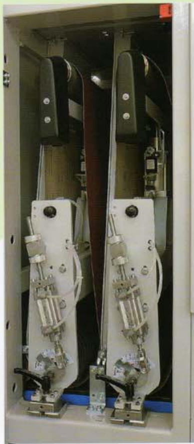
2RR - 2 Schleifaggregate 2RR - 2 Belts units
